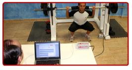
This device displays and registers relevant biomechanical parameters (displacement, velocity, acceleration, force, power, ...) of most weight-lifting exercises performed in a vertical plane against a constant load. Data such as peak force, mean velocity, mean power, time to peak power, propulsive phase's duration, etc. are automatically computed and presented on screen, both numerically and graphically.
